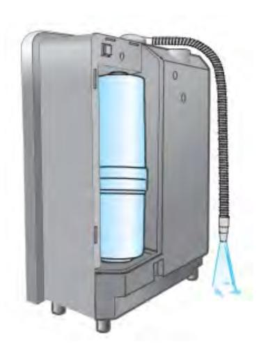
Now switch the main switch ON again, open the water supply with the turn dial and test the new filter to see if it is sealed for 2-3 minutes.
